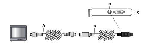
**NOTE:** The S-video adapter cable is only needed if there is no composite video jack on the back of the PC.
